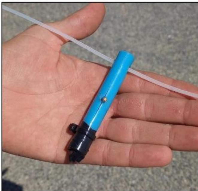
Figure 11-3. View of acoustic transmitter installed horizontally in a plastic protective tube for range testing exercises.
