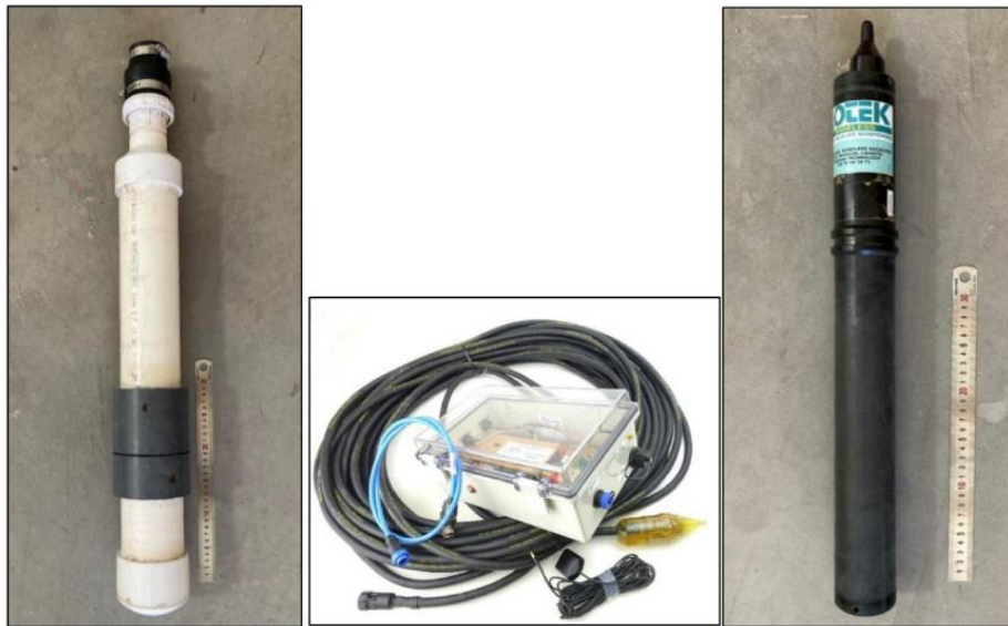
Figure 11-1. ATS (SR3001 on left and SR3017 in center) and Lotek (WHS 4250 on right) hydrophones. Reference ruler is 30 cm.
