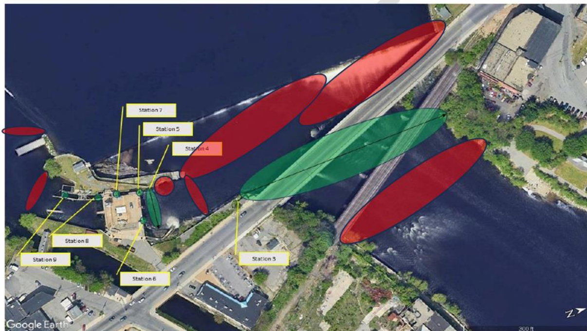
Figure 6-2. Proposed stationary receiver placement for monitoring upstream passage effectiveness at the Lawrence Project
