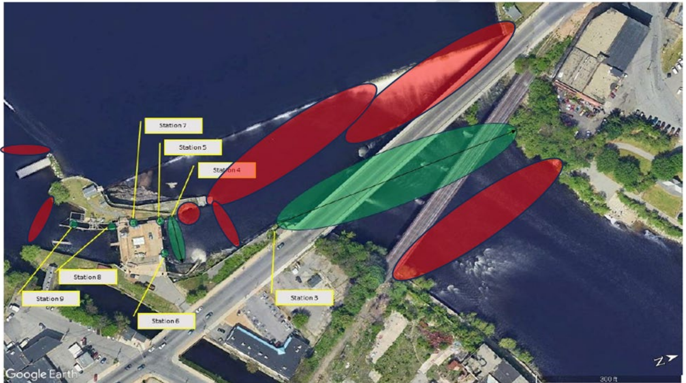
Figure 6-2. Proposed stationary receiver placement for monitoring upstream passage effectiveness at the Lawrence Project
