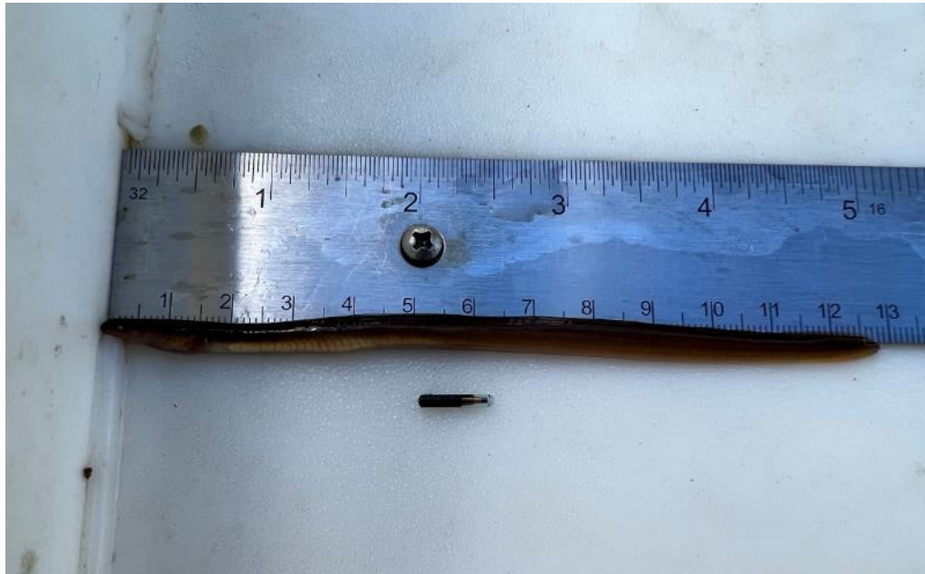
Figure 7-1. Oregon RFID 12 mm HDX PIT tag and a 128 mm juvenile American eel
