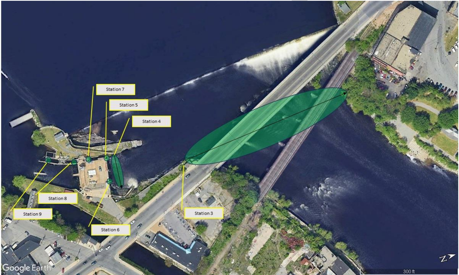
Figure 6-2. Proposed stationary receiver placement for monitoring upstream passage effectiveness at the Lawrence Project
