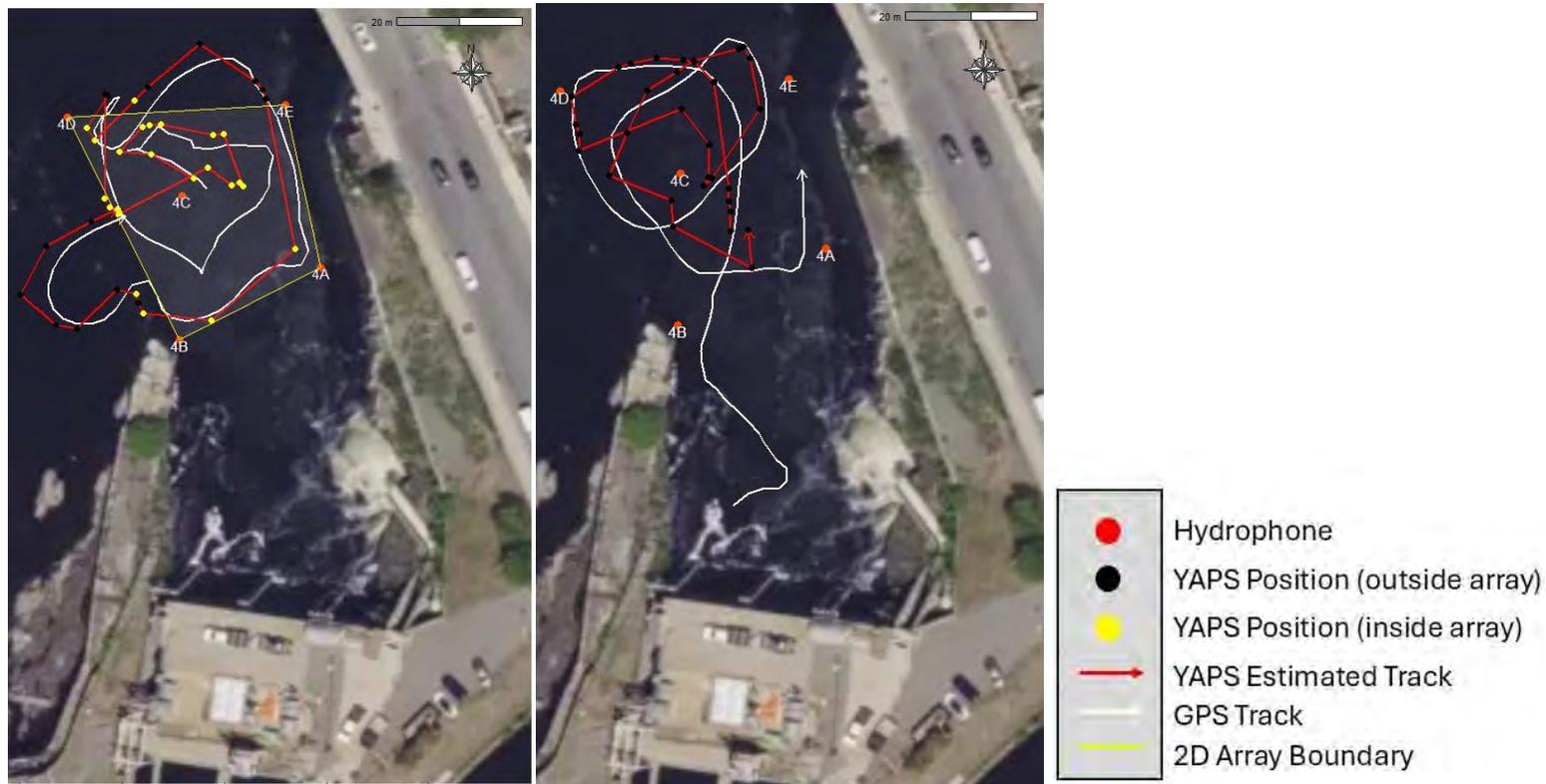
**Figure 5-7. Test transmitter position and resulting YAPS positional estimates for the ATS SS300 tag during two transmitter tests at pilot deployment location 4 during Phase 1 of the Project Interaction Study at Lawrence. YAPS positions are identified as those associated with GPS/transmitter track within the boundary of the targeted 2D detection area (yellow) and those associated with GPS/transmitter track outside the boundary of the targeted 2D area (black).**
