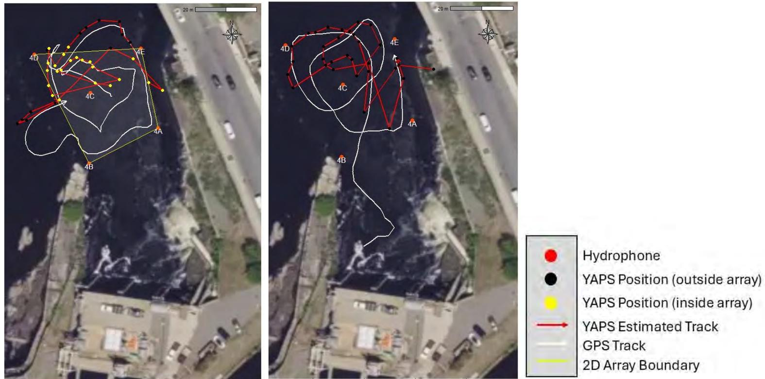
**Figure 5–8. Test transmitter position and resulting YAPS positional estimates for the ATS SS400 tag during two transmitter tests at pilot deployment location 4 during Phase 1 of the Project Interaction Study at Lawrence. YAPS positions are identified as those associated with GPS/transmitter track within the boundary of the targeted 2D detection area (yellow) and those associated with GPS/transmitter track outside the boundary of the targeted 2D area (black).**
