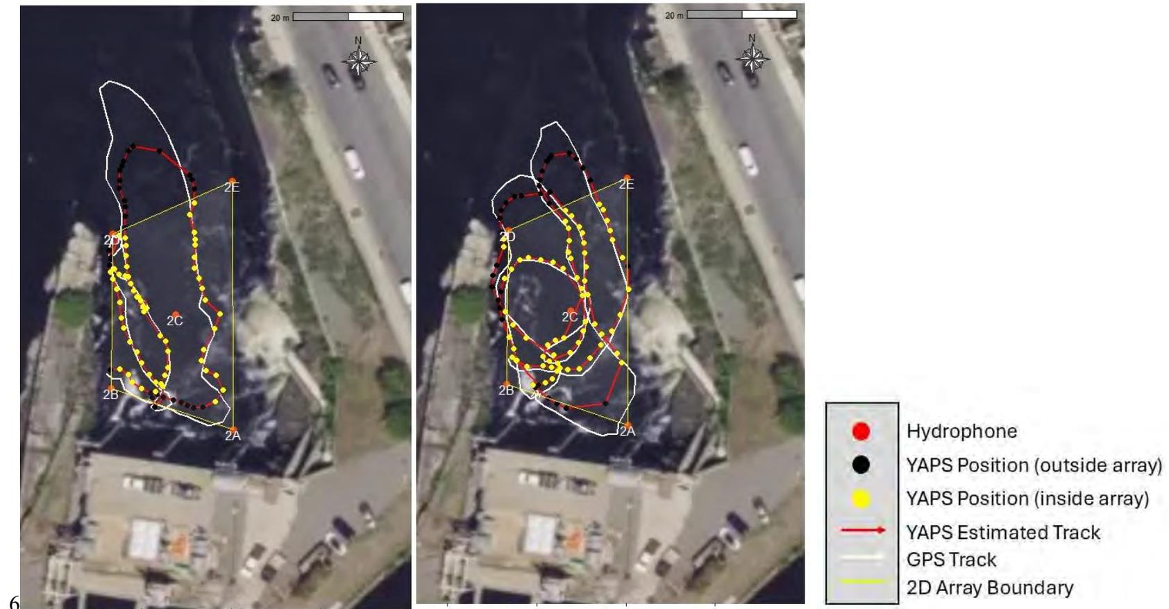
**Figure 5-5. Test transmitter position and resulting YAPS positional estimates for the ATS SS400 tag during two transmitter tests at pilot deployment location #2 during Phase 1 of the Project Interaction Study at Lawrence. YAPS positions are identified as those associated with GPS/transmitter track within the boundary of the targeted 2D detection area (yellow) and those associated with GPS/transmitter track outside the boundary of the targeted 2D area (black).**
