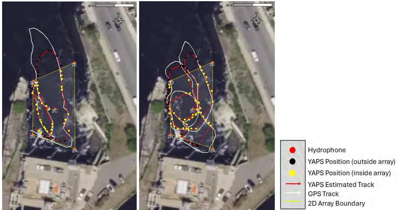
**Figure 5-4. Test transmitter position and resulting YAPS positional estimates for the ATS SS300 tag during two transmitter tests at pilot deployment location #2 during Phase 1 of the Project Interaction Study at Lawrence. YAPS positions are identified as those associated with GPS/transmitter track within the boundary of the targeted 2D detection area (yellow) and those associated with GPS/transmitter track outside the boundary of the targeted 2D area (black).**
