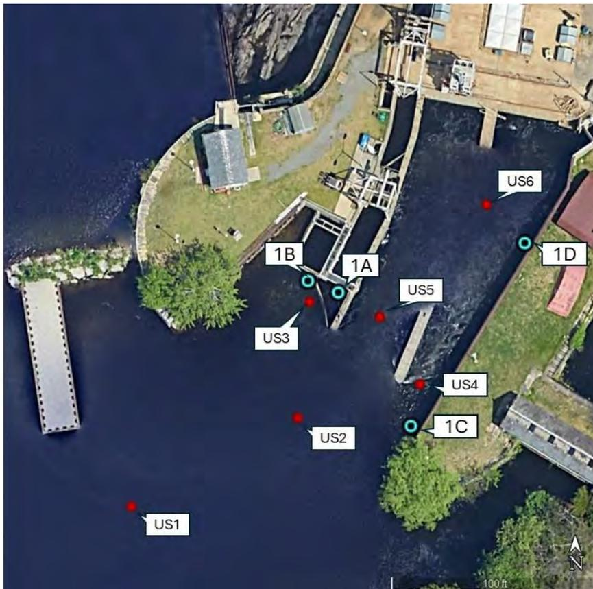
**Figure 5–2. Receiver (1A-1D) and transmitter (US1-US6) placement during field evaluation at pilot deployment location 1 during Phase 1 of the Project Interaction Study at Lawrence.**
