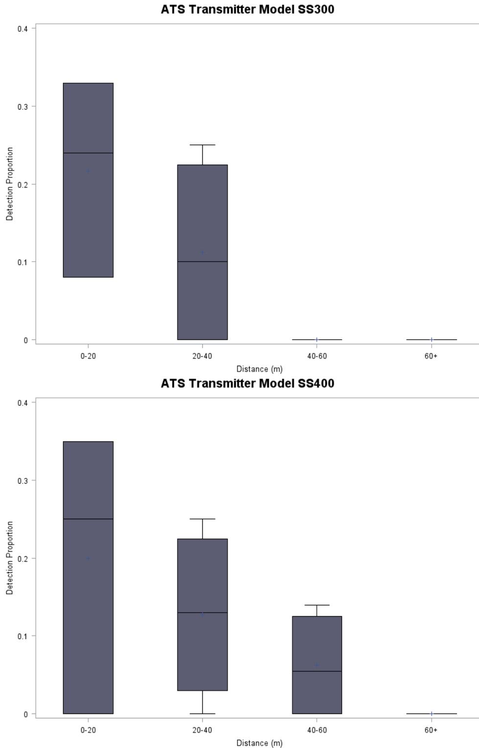
**Figure 5–11. Observed detection rates for the SS300 (upper panel) and SS400 (lower panel) transmitters by ATS receivers installed at pilot deployment location 5 during Phase 1 of the Project Interaction Study at Lawrence.**
