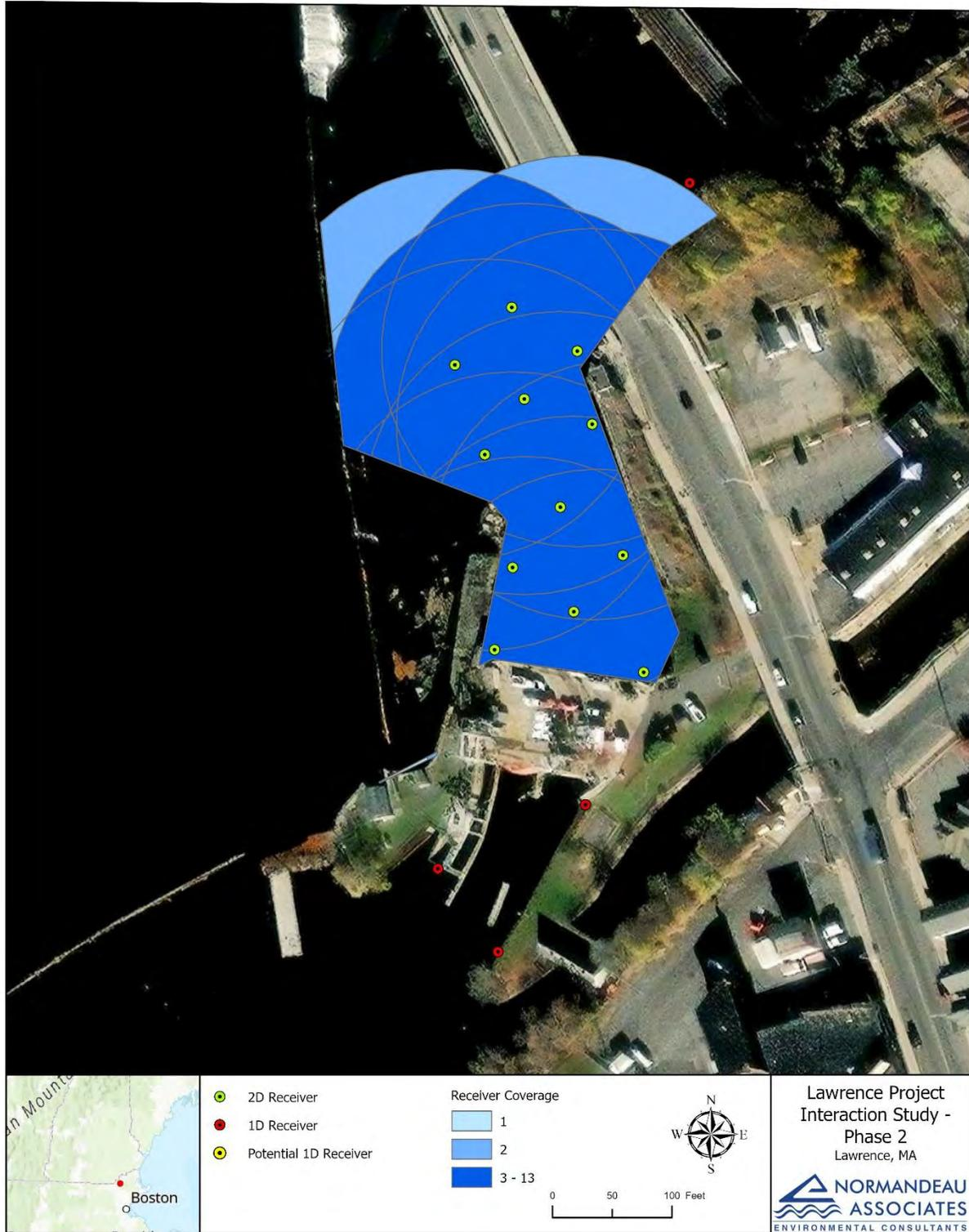
**Figure A-1. Proposed acoustic receiver installation for the 2D component of the Project Interaction Study at Lawrence.**
