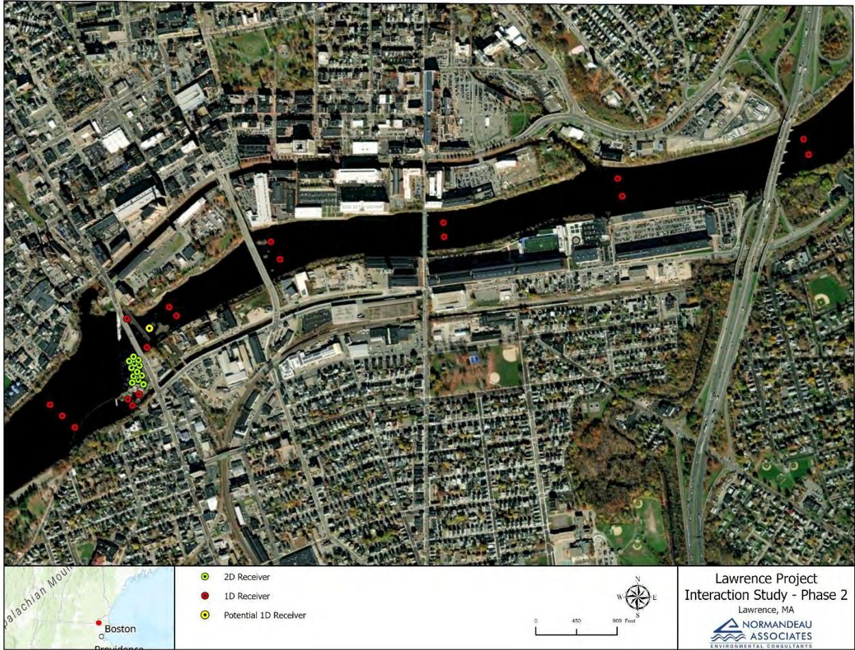
**Figure A-2. Proposed acoustic receiver installation for the 1D component of the Project Interaction Study at Lawrence.**
