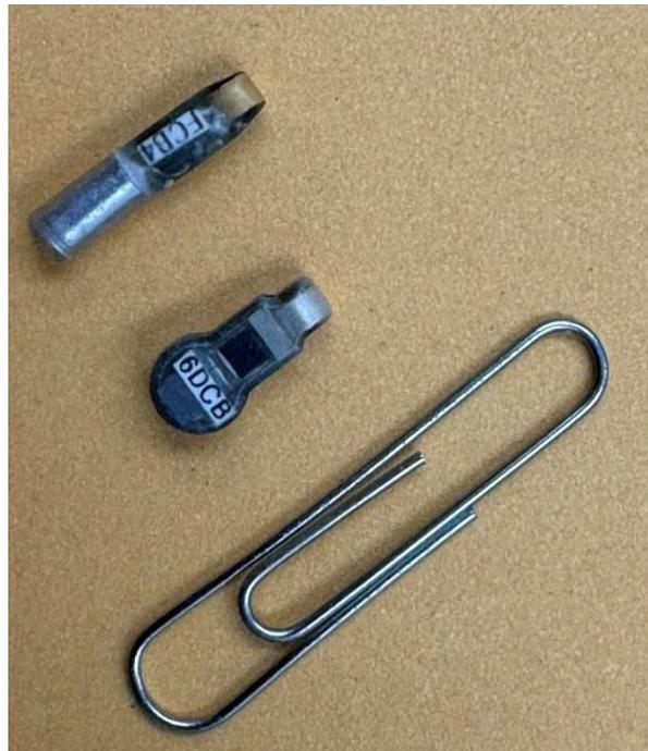
**Figure 4–1. JSATS SS300 (lower) and SS400 (upper) transmitters manufactured by ATS and used in the river herring tag retention and survivability assessment as part of Phase 1 of the Project Interaction Study at Lawrence.**
