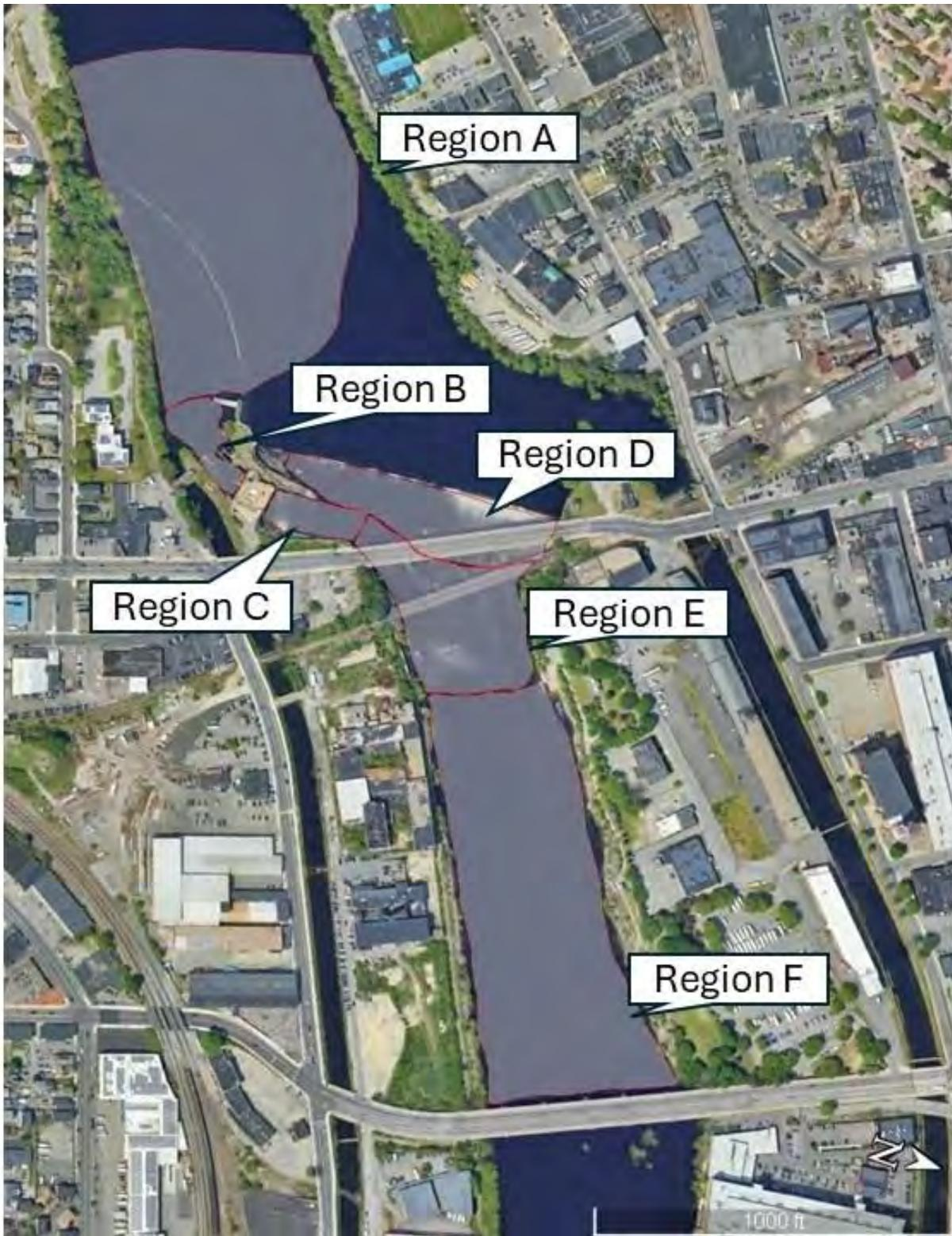
Figure 6-1. General regions based on hydraulic and bathymetric conditions in the vicinity of the Lawrence Project.
