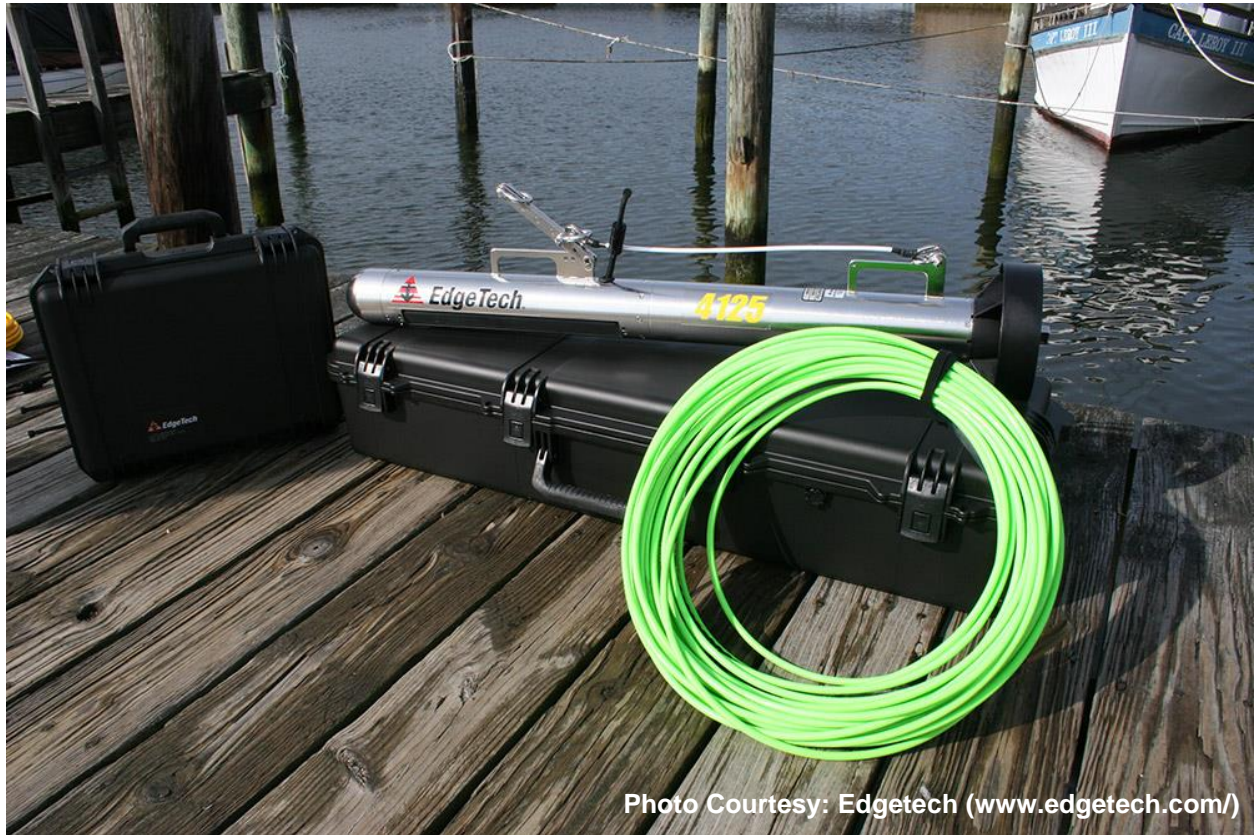
Figure 1-1. Photo of the Edgetech 4125i 600/1600 kHz side-scan sonar (SSS) with cable and topside processor to be used in the mobile SSS survey.
