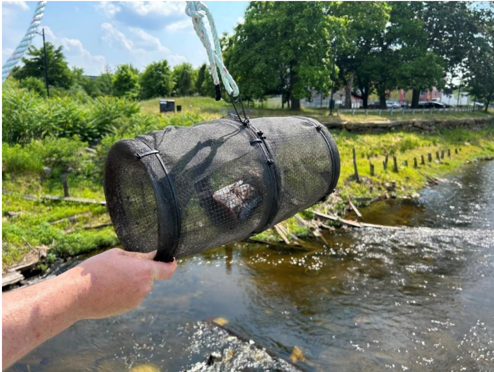
Figure 4-10. Modified minnow pot lined with reduced size mesh and baited for the collection of juvenile eels in the vicinity of the Lawrence Project.
