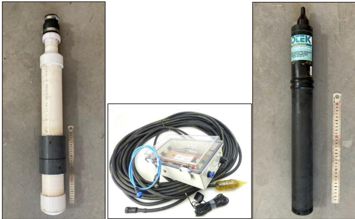
Figure 3: ATS hydrophone (SR3001 on the left and SR3017 in the middle) and Lotek WHS 4250 hydrophone to the right. The reference rule is 30 cm.
