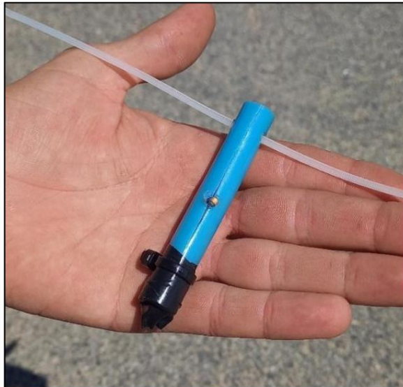
Figure 4: view of a transmitter installed horizontally in a plastic protective tube.
