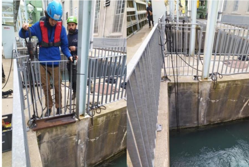
Figure 6: Positioning of the LOTEK and ATS hydrophones on a double rope stretched by a piece of railway rail, along the wall of groups 2 and 3.
